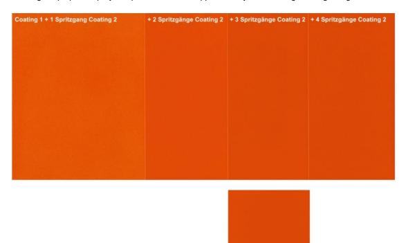
The painter can now inspect visually and identify the colour that matches the best with the original finish. In our example, it's the sample number 3 with 3 layers of "Coating 2".
